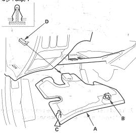
2. Install the cover in the reverse order of removal, and push the clip into place securely.
