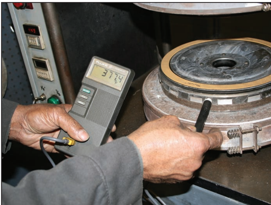
Figure 5: Never trust the temperature dial on your bonding press; check the temperature directly using a digital pyrometer, to make sure the clutch is reaching bond line temperature.
