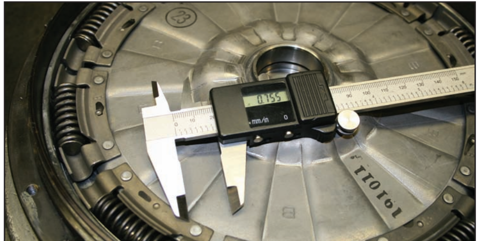
Figure 9: Next, lay the clutch into place, and measure the height from the top of the clutch assembly (where it rides on the clutch release stop on the turbine) to the bearing surface.
