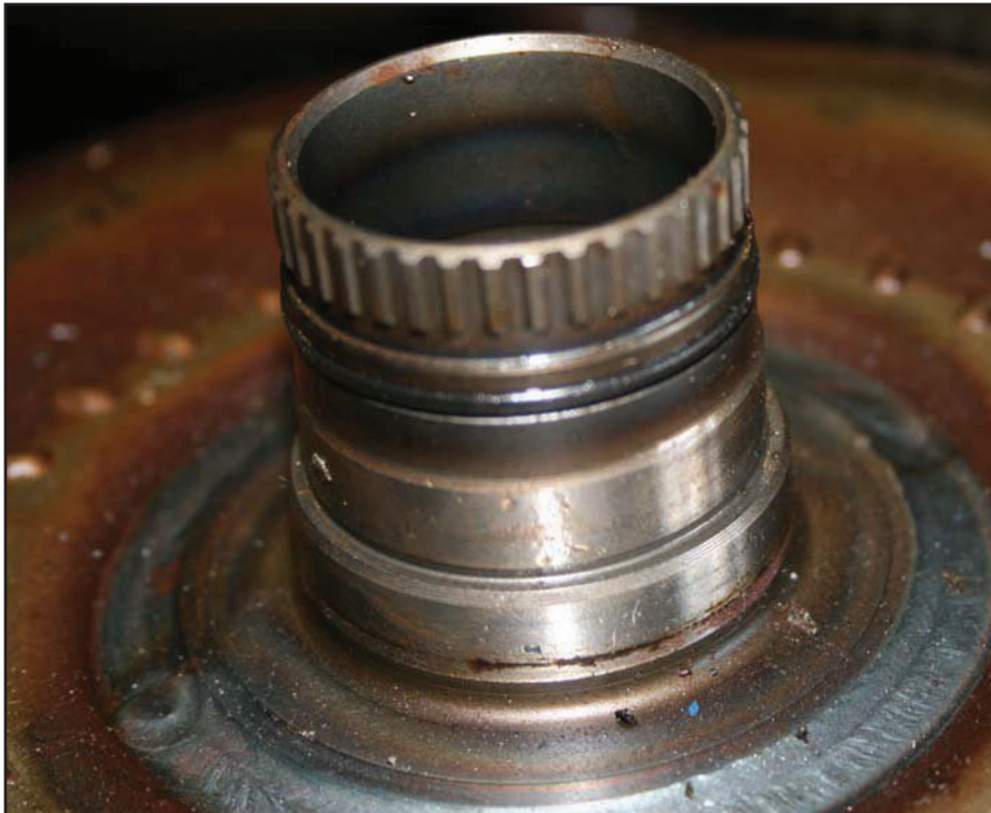
Figure 2: The black O-ring worked fine when the transmission was new, and none of the components were worn. But over time the combined component wear can allow the black O-ring to leak.
