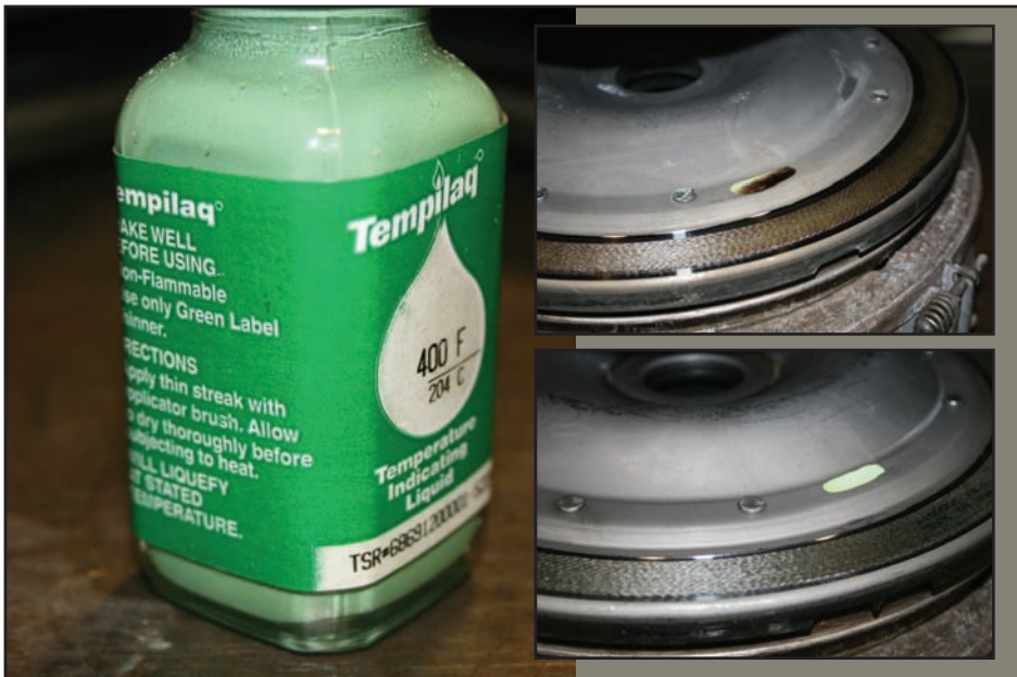
Figure 7: Another easy way to monitor the clutch bond line temperature is to use a Tempilaq to mark the clutch piston. If the mark changes color, you can be sure the piston reached the temperature necessary for a proper bond.
