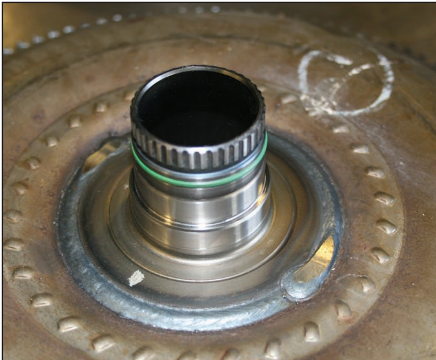
Figure 3: Always replace the black O-ring with the new, green O-ring. The green O-ring is thicker, so it compensates for small amounts of wear in the different components, providing a good seal.
