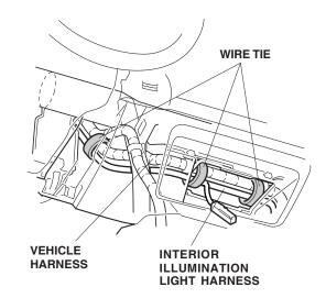
24. Secure the interior illumination light harness to the vehicle harness using four wire ties if the vehicle is equipped with the driver's dashboard under cover. Use three wire ties if the vehicle is without the driver's dashboard under cover.
