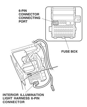
NOTE: If another accessory is already plugged into the 6-pin connector, remove the dummy connector from the other accessory harness, and plug the interior illumination light harness into that connector.
