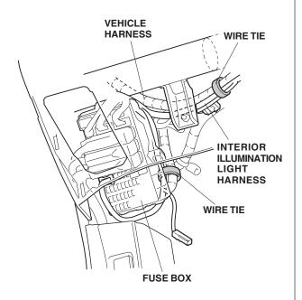
23. Secure the interior illumination light harness to the vehicle harness with three wire ties.
