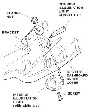
32. Bundle the interior light harness and secure the connector to the bracket using a wire tie with clip.
