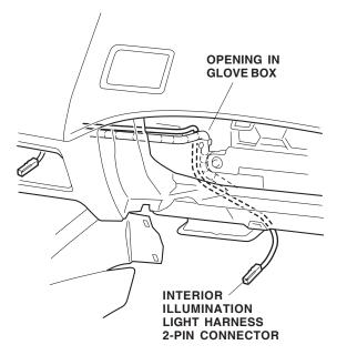
22. Secure the interior illumination light harness to the vehicle harness with two wire ties.
