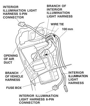
12. Measure the vehicle harness from the point of branch as shown. Secure the interior illumination light harness (6-pin connector side) to the vehicle harness with one wire tie.
