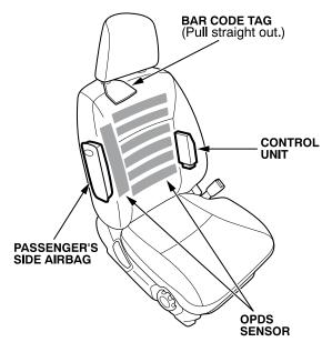
NOTE: If the seat gets wet from rain or spilled liquids, the SIDE AIRBAG indicator may come on. If this happens, dry the seat, and the indicator should go off.
