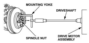
Set the lower toggle switch on the drive motor assembly to FWD (counterclockwise rotation) or REV (clockwise rotation).
