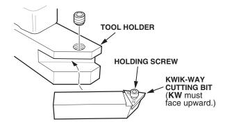
Before you use the brake lathe, inspect the tips of the cutting bits with a magnifying glass to make sure the tips are not worn out. Each bit has three tips. If a tip is worn, rotate the bit, and use a new tip. A worn tip will produce a poor finish and may cause chattering.
