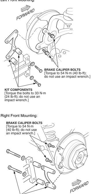
**KIT COMPONENTS** [Torque the bolts to 33 N·m (24 lb-ft); do not use an impact wrench.]
