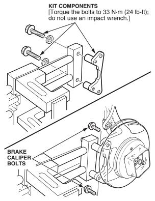
[Torque to 54 N·m (40 lb-ft); do not use an impact wrench.]
