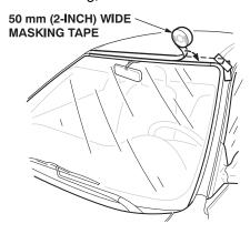
2. Pull the rear edge of the upper windshield molding away from the roof (use a cotter pin puller or similar tool), and apply a liberal amount of 3M Black Super Silicone Sealant underneath it. Apply sealant along the entire masked-off area.
