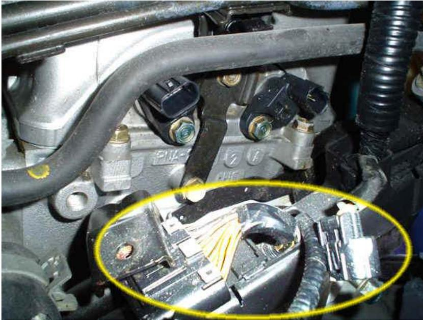
Lift up this plastic and it will reveal the radiator coolant temp sensor
