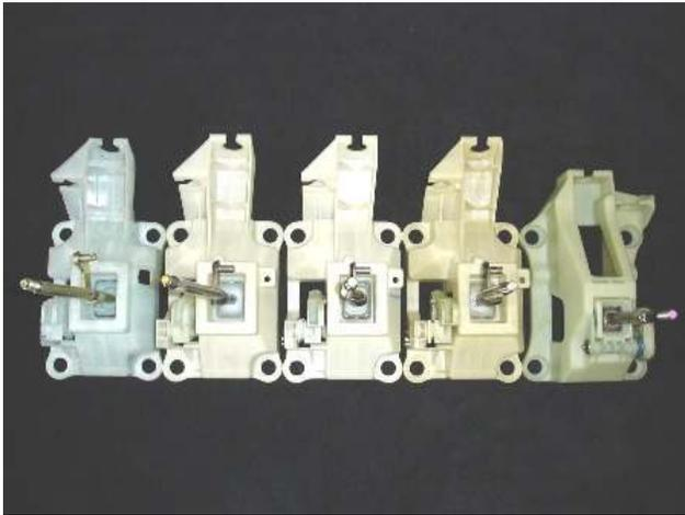
The Revo, RSX-S, Base RSX, and 01+ Civic (Non-Si) can all shift the 6 speed tranny, including reverse. The TSX shifter may be a different design but still bolts up to the same place as the other shifters and functions just as same. It can even use the same short shifter adapters as the other shifters.
