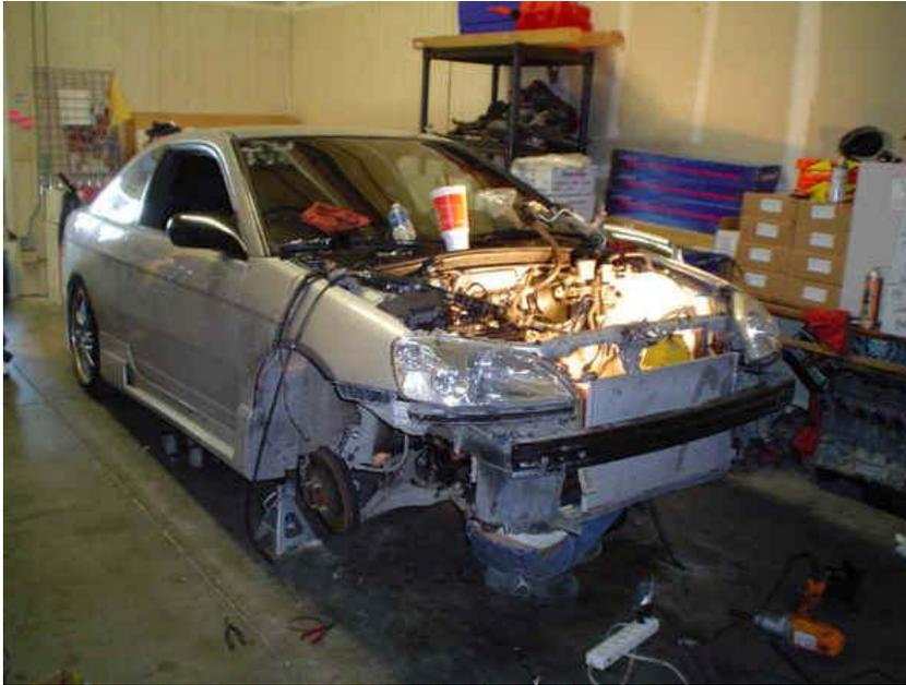
Now if you pulled the motor from the top. Jack the car back up so you have enough space to pull out the subframe. There are 4 bolts holding up your subframe. Take those 4 bolts out and the whole thing will drop.
