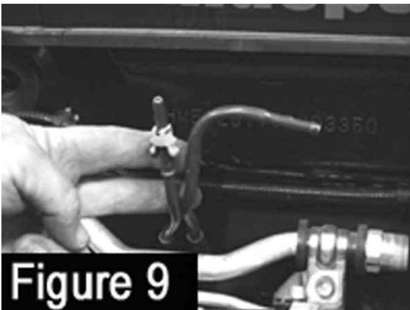
You have to gently bend the lines so that way it bends with the right line facing to the right and the left line is pointing towards the front of the engine bay. Now if you want to label these lines the left is the FUEL and the right one with the bend is the PURGE which hooks up to a vacuum on the manifold. Make sure you make no kinks in these lines or
