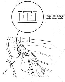
3. Test the motor in each direction by connecting battery power and ground according to the table. When the motor stops running, disconnect one lead immediately.
