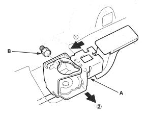
Disconnect the trunk lid opener/fuel fill door opener cable (A), then remove the opener (B). Take care not to kink the cable.
